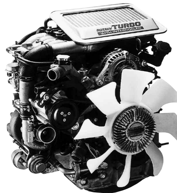
13B Rotary Turbo Engine ■ The second generation RX-7 made its debut in 1985, featuring a 13B rotary engine boosted by a Twin-Scroll Turbo. The engine produced a maximum output of 185PS.
